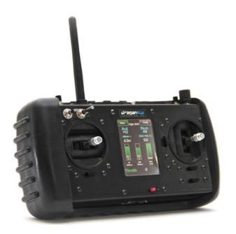
The Draganfly custom designed Handheld Controller features a direct sunlight viewable touch screen and most importantly every switch or button has a purpose. The controller is ergonomically designed to provide precise helicopter control. The controller is compatible with all Draganfly series helicopters. As an add-on option illustrated below, the controller can be fitted with a Nexus digital video display for use with any Draganfly aircraft utilizing a digital video payload.
