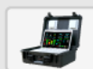
Wireless Video Base Station with Quad Diversity Video Receiver and Video Capture Device
