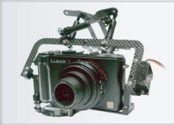
10.1MP Digital Camera with 720p HD Video, Anti-Vibration Mount, and SD Wireless Video Transmitter
