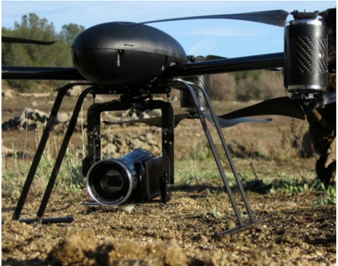
The Draganflyer X6 is a six motor electric powered UAV helicopter capable of carrying a wide range of camera payloads.
