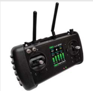
Handheld Controller with Touchscreen Display and Wireless Video Receiver
