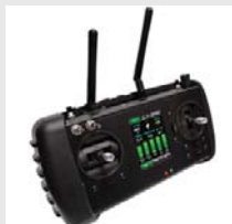
Handheld Controller with Wireless Video Receiver and OLED Display
