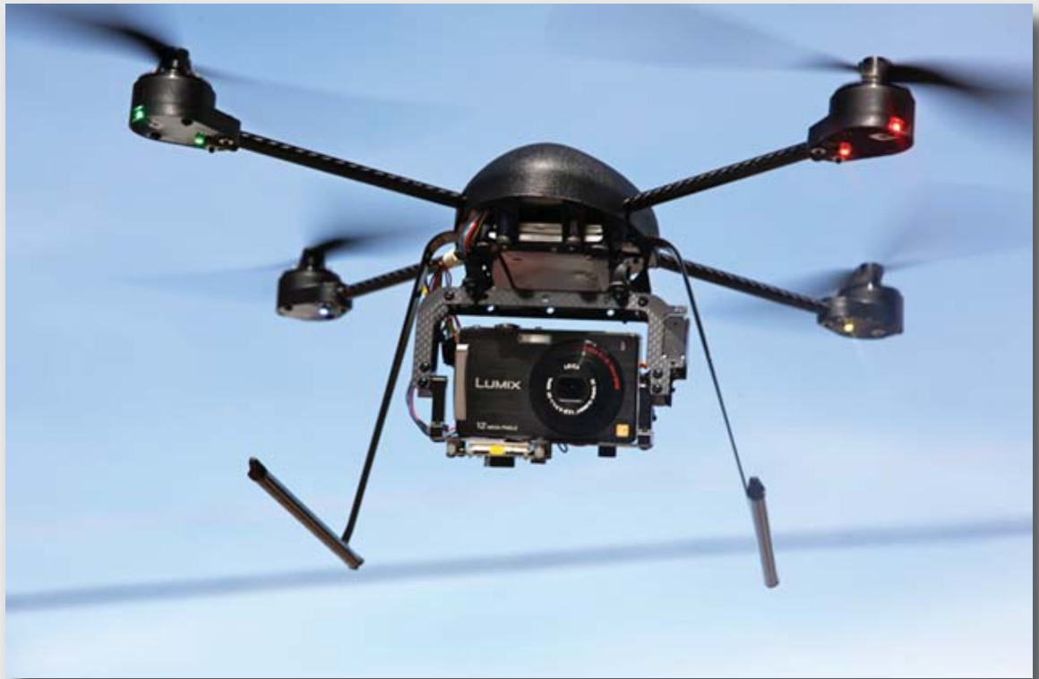
12.1MP Digital Camera with 720p HD Video, Anti-Vibration Mount, and SD Wireless Video Transmitter
