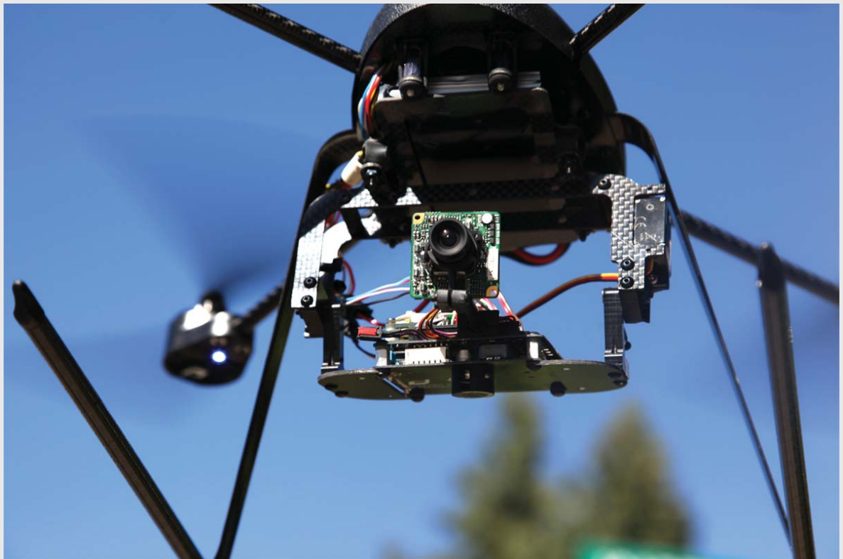
Low Light Video Board Camera with Anti-Vibration Mount, Wireless Video Transmitter and Onboard Digital Video Recorder
