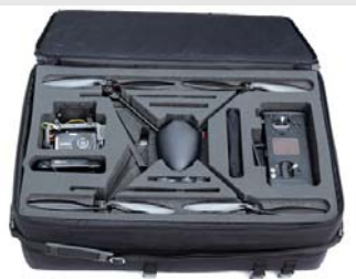
Draganflyer X4 Softpack made from high density foam and nylon allow all the Draganflyer X4 parts and components to fit neatly in the transport case
