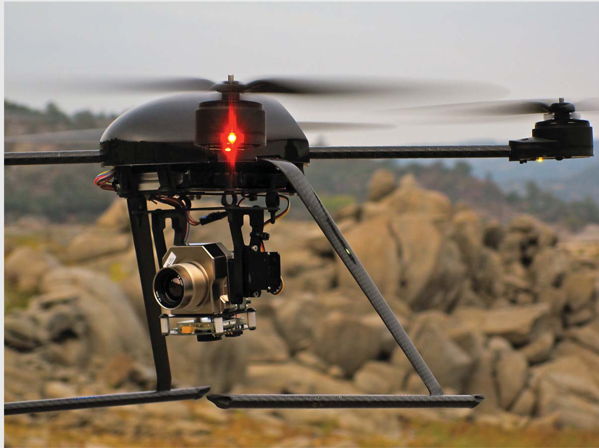
Thermal Infrared Video Camera with Anti-Vibration Mount and Wireless Video Transmitter
